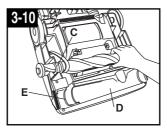
Insert agitator through belt and place belt in belt guide (C) on agitator.
